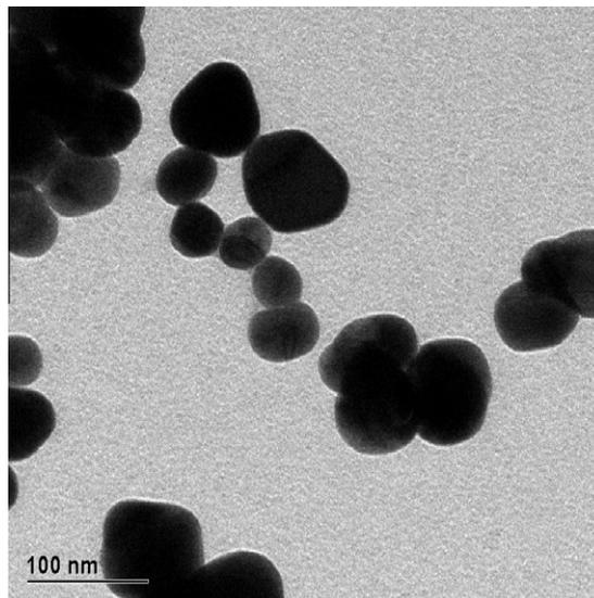
Fig. 2. Transmission electron micrograph of nano-Ag.
