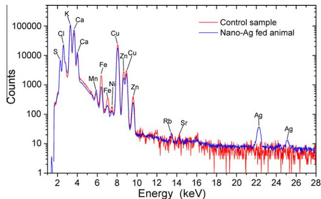
Fig. 4. Micro-PIXE spectrum measured by germanium X-ray detector on the section of digestive gland tissue: control sample and nano-Ag fed animal.
